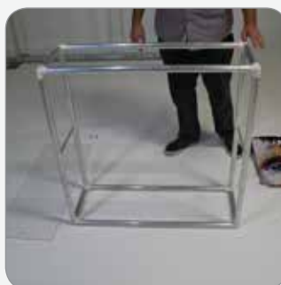
5. Find the holes located on the sides. This is for mounting the top piece.
