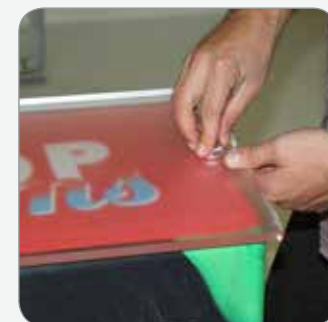
9. Connect the top piece with the two provided bolts.
